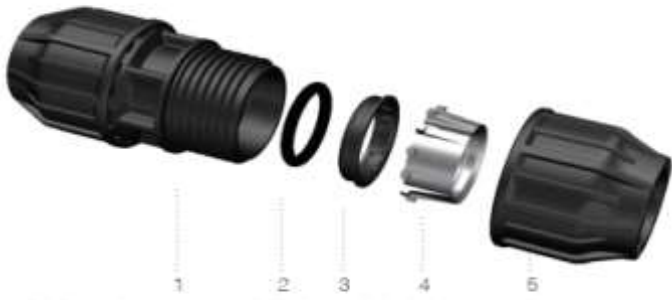
1. BODY - Polypropylene PP-B / 2. O-RING - Nitrile Rubber (NBR 70) / 3. INSERT - Polypropylene PP-B / 4. SPLIT RING - Polyacetal / 5. NUT - Polypropylene PP-B
