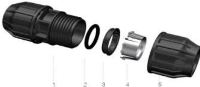
1. BODY - Polypropylene PP-B / 2. O-RING - Nitrile Rubber (NBR 70) / 3. INSERT - Polypropylene PP-B / 4. SPLIT RING - Polyacetal / 5. NUT - Polypropylene PP-B
